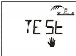
This function tests all the stations connected to the controller using a 2-minutes cycle and allows you to check that your irrigation system is working properly.
