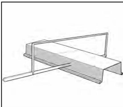
The gutters have to be cut in the correct length. PVC gutters can be cut easily with a small saw. Make sure the cut is straight and clean. If necessary, you can clean the cut with a knife or a piece of sandpaper. Also wipe off remaining sawdust from the gutter.
