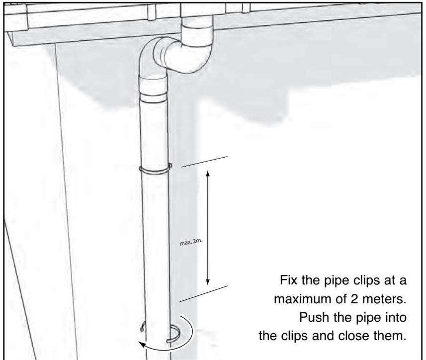
Fix the pipe clips at a maximum of 2 meters.
