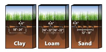
These illustrations show water movement in a sub-surface application. These guidelines apply to on-surface as well as sub-surface installations.
