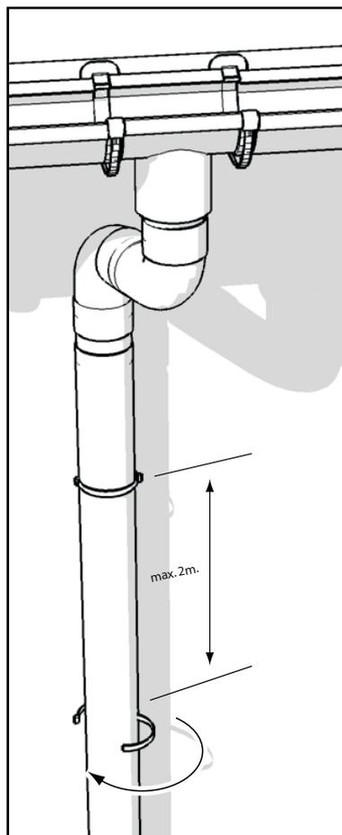
Fix the pipe brackets at a maximum of 2 meters. Push the pipe into the brackets and close them.
