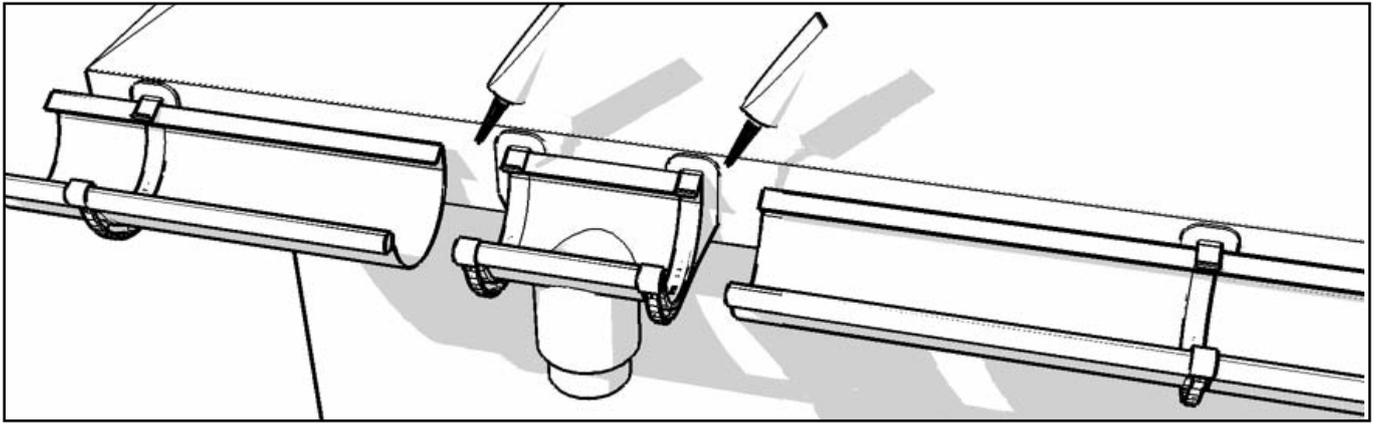
If you use glue-fittings, the gutter can be glued into the fittings. Make sure the surface is clean before applying the glue. The seam in which the gutter is stuck, must be filled with glue. Afterwards, apply some additional glue along the inside seam.
