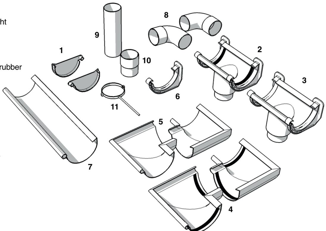
Determine the position of the outlet. That is automatically the lowest point. After that, you can also determine the highest point. Install a bracket at the lowest and one at the highest point. A string secured between both brackets will assist in installing the remaining hangers.
