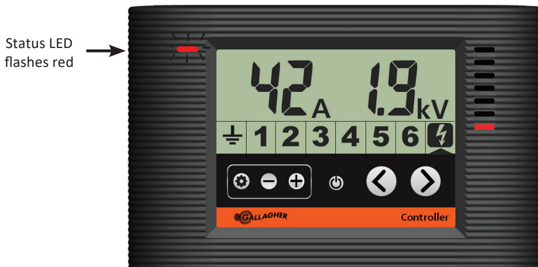
Controller showing the energizer in output alarm
