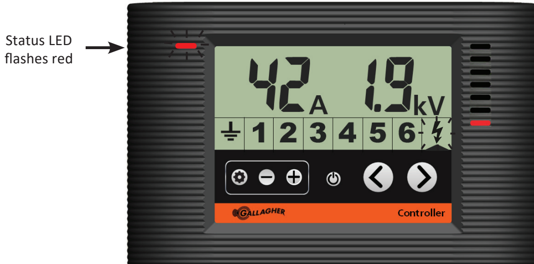
Controller showing the energizer in current alarm
