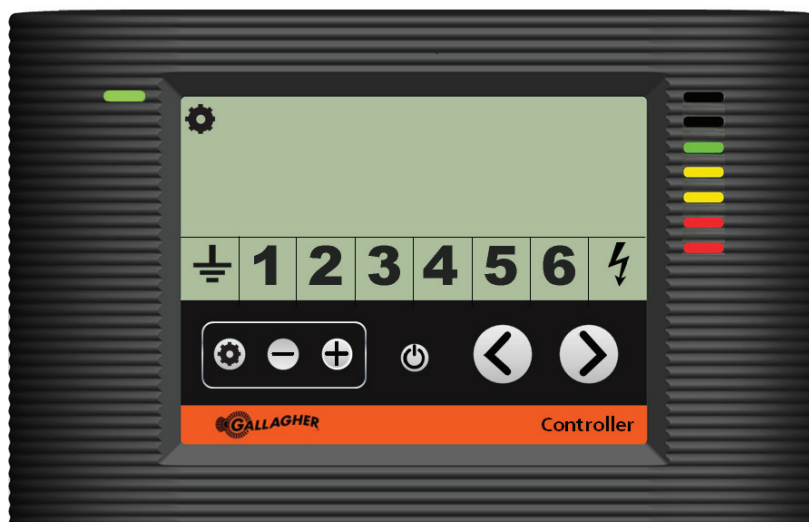
Controller showing the output voltage being adjusted
