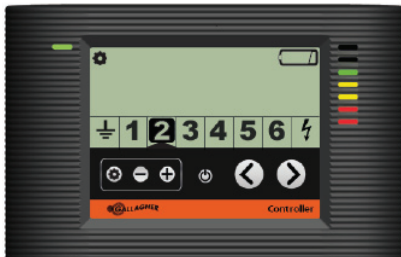
Bedieningspaneel toont zone 2 met lege batterijen
