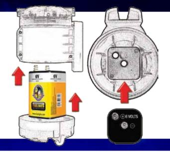
Powered by a 6 volt battery (which is not included) placed into the unit with the 2 terminals making contact trhough the holes in the top of the power board.
