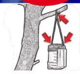
With a strong tie to a beam or tree branch. (Note the tree trunk will obscure the light in its direction)
