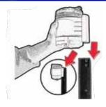
The preferred method to mount your Foxlights is on the back of a star post placed in position to maximize field coverage.
