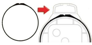
To insure waterproofing, keep both rubbel seals positioned correctly on top and bottom of the unit.
